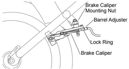
To tighten the cable, loosen the lock ring and turn the barrel adjuster in the counter clockwise direction. Secure the barrel adjuster in the new position by tightening the lock ring against the caliper or brake lever body.
