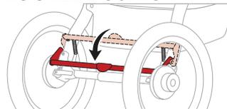
To ensure the brake is set properly, attempt to roll the stroller fore and aft after setting the brake. If the stroller will not roll, the brake is set properly.
