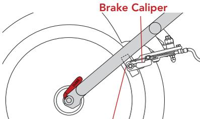
Brake Pad Aligned With Rim
