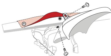
NOTE: You might want to remove a fabric screw (right or left) to give better access to the cross tube mounting hole.
